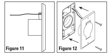
Align the inlet screw holes with the mounting plate holes and press the inlet into place, guiding any extra wire back through the mounting plate as you go. Attach wall inlet to mounting plate with provided screws (Figure 12).
